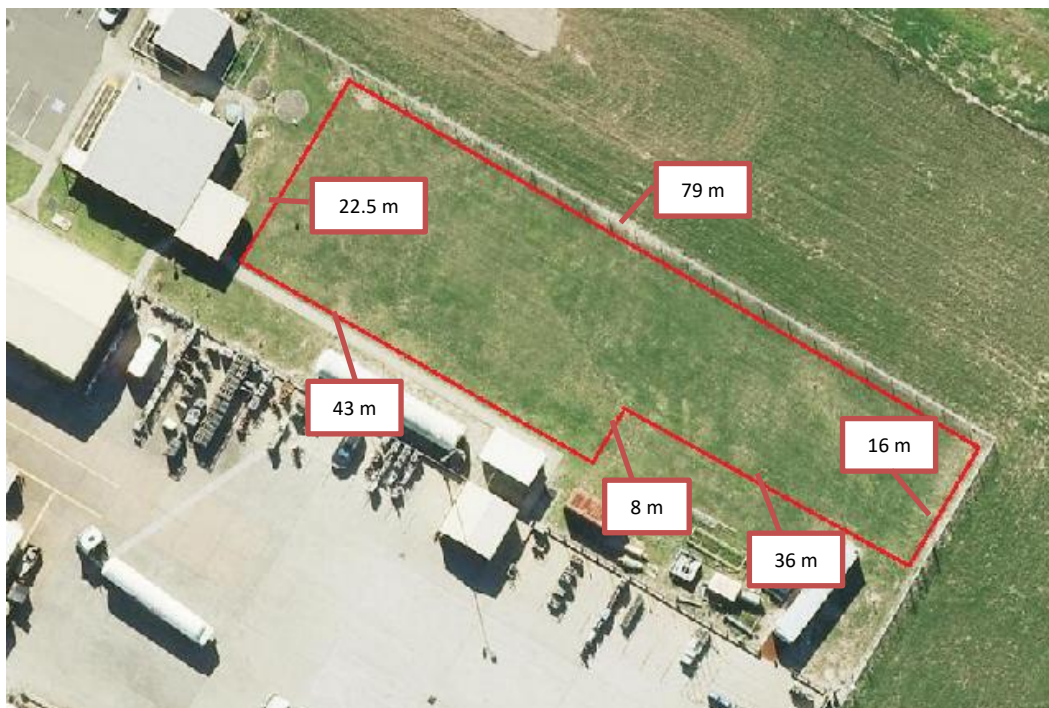
Figure 3.1: Grassed area for irrigation of cooling tower effluent
