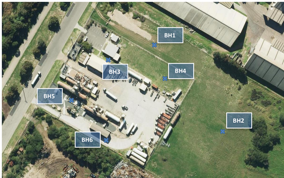
Figure 4-2: Location of groundwater monitoring bores BH1 to BH6
