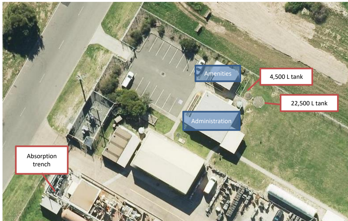
Figure 3.4: Septic system and absorption trench locations
