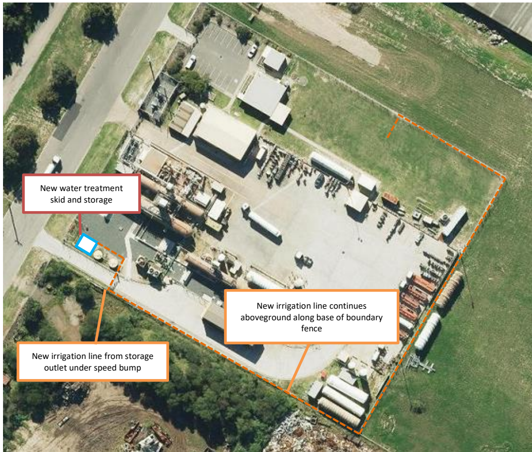
Figure 4-3: Proposed revised irrigation pipework system diagram
